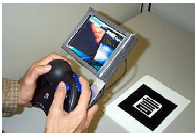
Figure 6: AR Pad: Interaction tool and display combined in one device. (after [4])
