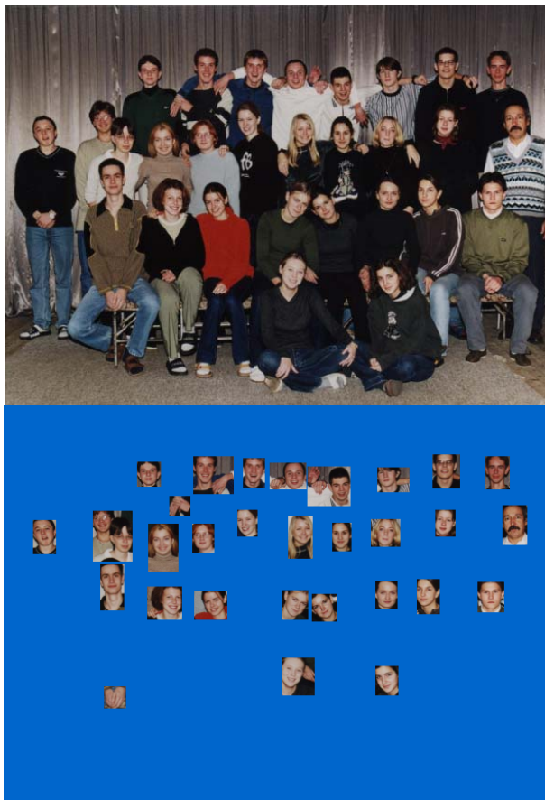
Figure 19: Image processing using MG/hsv skin-color model, Assumptions A, B, C and without pre-filtration
