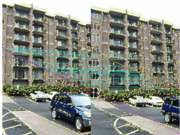
Figure 10 : Guided matching. Matching is processed on two corresponding epipolar lines.
