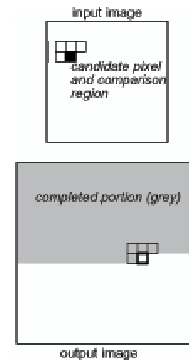
Figure 2: The new texture is generated pixel by pixel in scanline order. On each position, the algorithm identifies the corresponding L-shaped neighbourhood and searches for an equivalent one in the texture sample. As soon as it finds one, the pixel belonging to it is copied to the current position. The figure is taken from [3].
