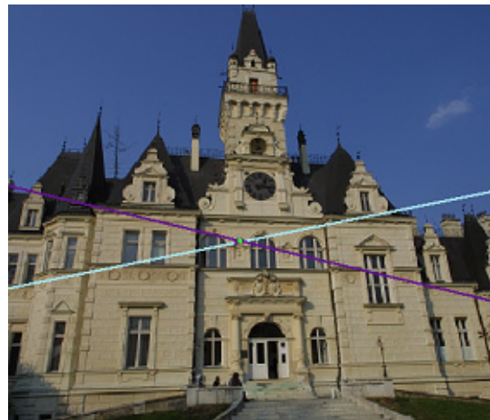
Figure 2: A light line is the epipolar line and a dark one is the false epipolar line. The corresponding point is located near their intersection.
