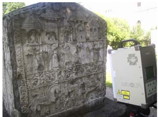
Figure 9. The Minolta 910 laser scanner is a scanner for close range and indoor applications and has an accuracy of under a millimeter.[2]
