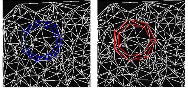
Figure 1: CDT in action. On the left we can see the proposed edges which should be constrained. On the right is the same TIN with constrained edges included.
