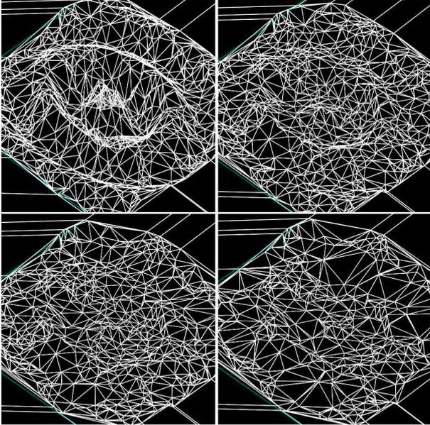
Figure 2: The automated simplification of the TIN. The top-left image shows the original TIN. The bottom-right image shows the simplified TIN which is more flat than the original due to erosion.
