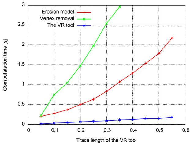
Figure 8: Time consumed by each part of computation in dependency on the trace length (the TIN size is 10000 vertices).
