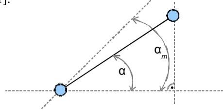
Figure 3: The material movement is stopped if an angle  $\alpha$  is less than the critical angle  $\alpha_m$ .
