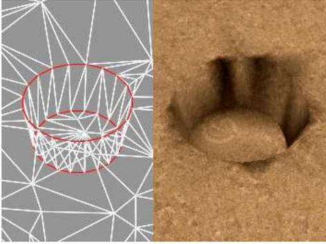
Figure 4: Stamping of a VR tool. On the left we can see the wire-frame model (red lines are constrained edges). On the right we can see the textured model. Both are without erosion; taken from [11].
