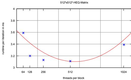
Figure 4: Dependence of the runtime of the number of threads per block.
