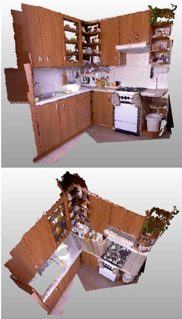
Figure 6: Reconstructed 3D model of the complex kitchen interior, based on 23 input frames. Resulting point clouds contains more than one million points and the reconstruction itself takes less than one minute to complete on the common today's hardware.
