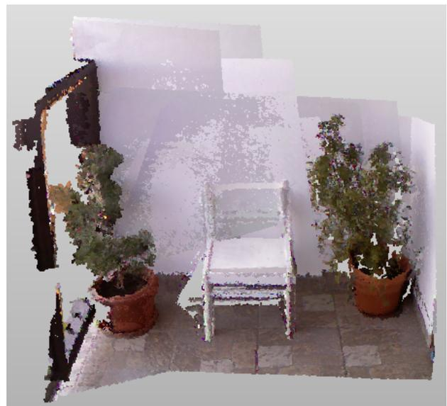
Figure 4: Reconstructed 3D model of the balcony scene. The irregularities of the wall color are caused by varying light conditions when capturing the individual frames.
