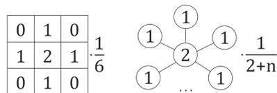
Figure 5: Left: convolution kernel of Gaussian blur for 2D digital image. Right: the same kernel for irregular graph.
