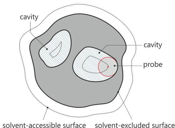
Figure 8: Illustration of cavity.
