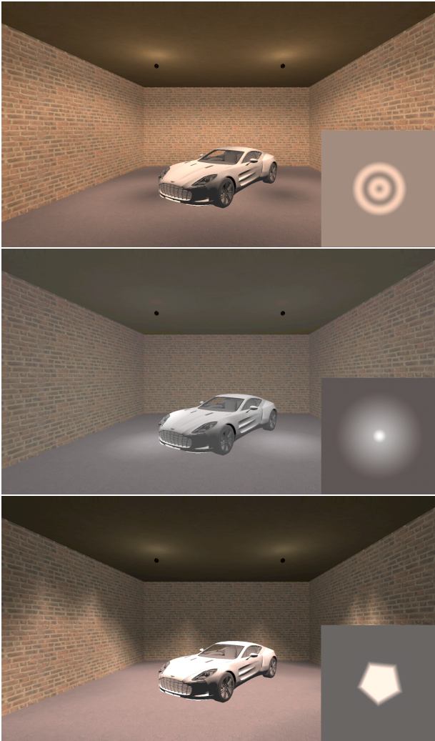
Figure 6: Renderings for different LDTs (shown in bottom right corner).
