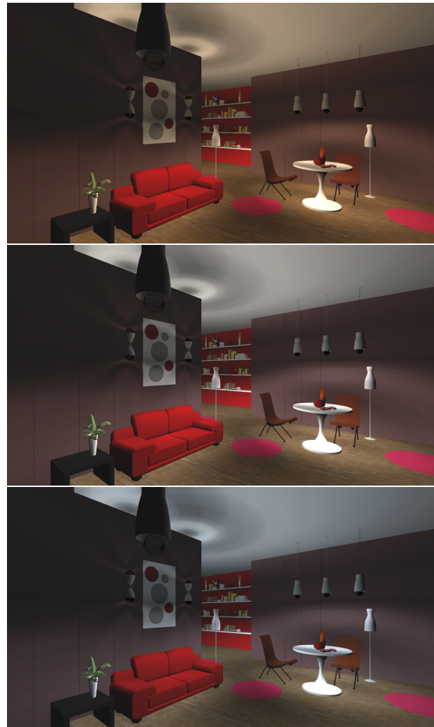
Figure 5: The same LDT with various colour temperatures (respectively from top to bottom image: 2850 K, 6000 K, 7000 K).
