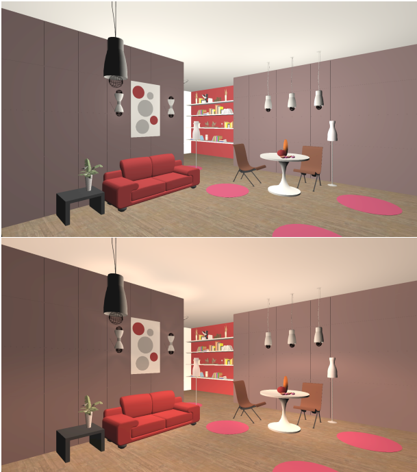
Figure 4: Typical point light model (top) and rendering based on goniometric light sources (bottom).
