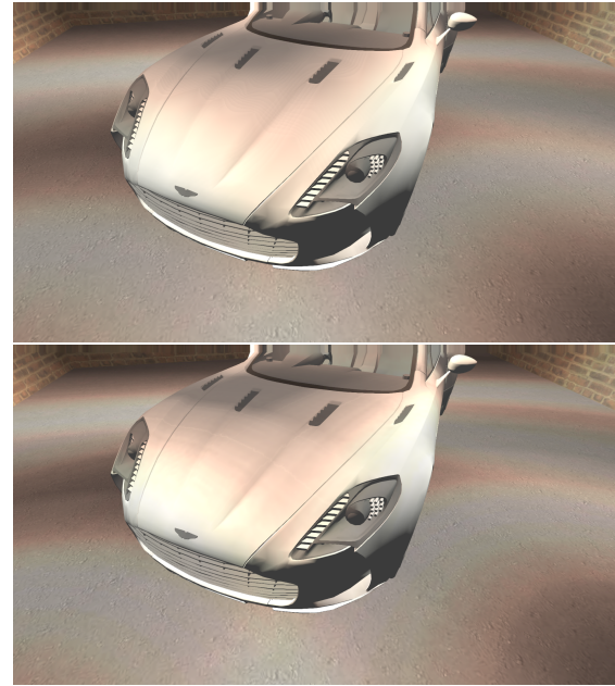
Figure 8: Images rendered with 2048x2048 pixels (top) and 128x128 pixels (bottom) LDTs.
