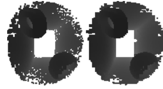
Figure 4: Example of an ISM with holes (left). The same ISM after 2 iterations of the pull-push algorithm fills small holes (right).
