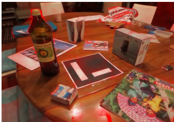
Figure 2: Visualization of the confidence map. Red shading denote regions with low confidence like, for example, the area around the bottle, which has been disoccluded due to the movement of the camera.
