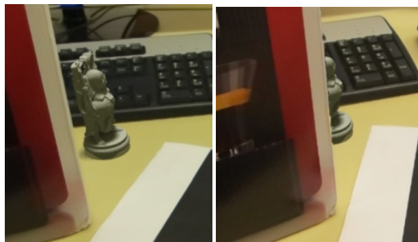
Figure 6: Occlusion of a virtual object (Buddha statue) by the real world using the estimated depth information.
