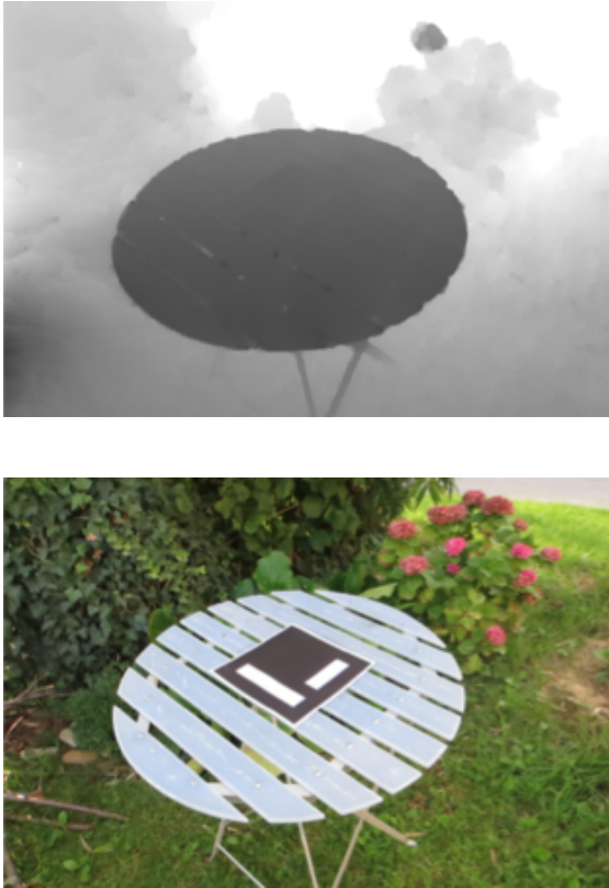
Figure 3: The top image shows the computed depth map for the reference image below.
