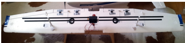
Figure 3: Camera rig mounted onto the wings
