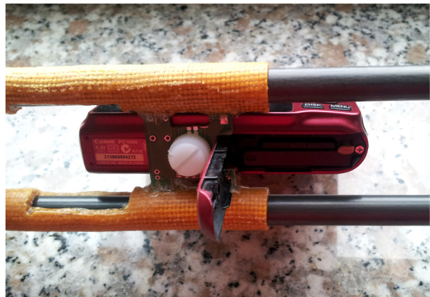
Figure 8: Camera cradle for the stereo rig
