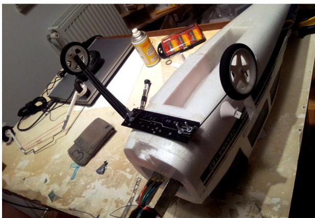
Figure 4: Carbon fiber landing gear with extended battery bay
