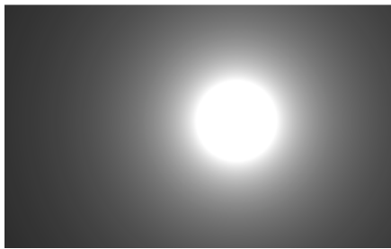
Figure 2: Region-of-interest mask computed based on CSF for an image of 1920x1080 pixel resolution (gaze position at (1000,500)), lighter area denotes higher frequency of HVS.
