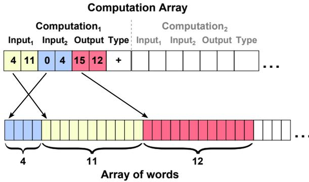
Figure 1: Memory layout of our numbers showing one example computation with two input and one output numbers as well as the operation type (+, −, ×) to be performed. The computation array holds the offset and size of the corresponding words in the global array of words.
