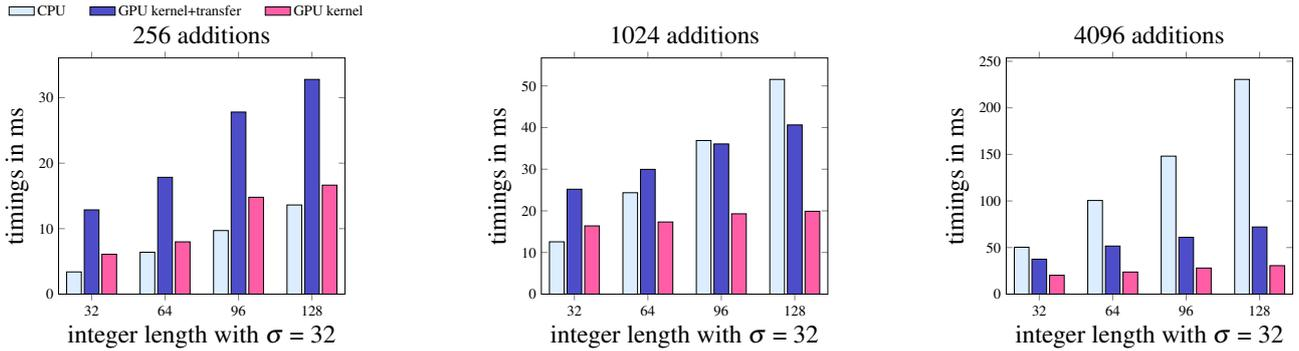
Figure 3: Addition benchmarks. Integer lengths in multiples of 1024 bits with deviation  $\sigma$  are shown on the x-axis. The timing of our GPU implementation is shown with and without data transfer to and from the device on the y-axis. For small computational loads, the GPU is not sufficiently occupied, while for a sufficiently large amount of computations, superior performance is obtained.
