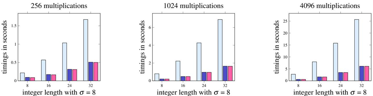
Figure 4: Multiplication benchmarks. Integer lengths in multiples of 1024 bits with deviation  $\sigma$  are shown on the x-axis. Due to the higher complexity of the multiplication, the GPU outperforms the CPU already at 256 multiplications and the advantage grows slightly as we raise the computation count.
