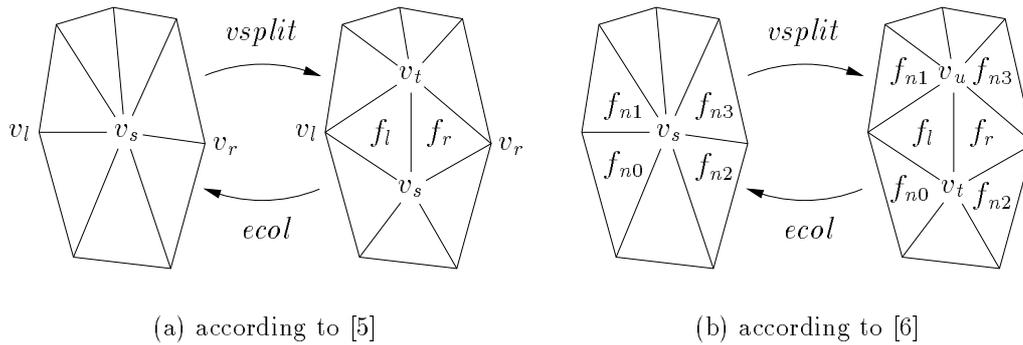
Figure 3: Different definitions of the mesh operations *vsplit* and *ecol*
