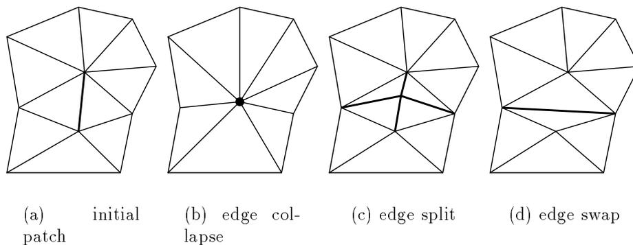
Figure 2: Local operations to modify the mesh connectivity
