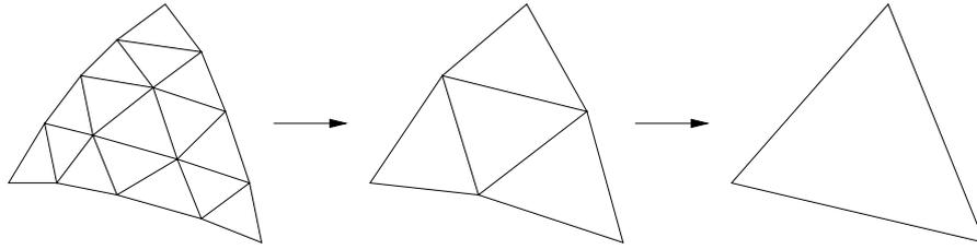
Figure 1: Simplifying a mesh with subdivision connectivity
