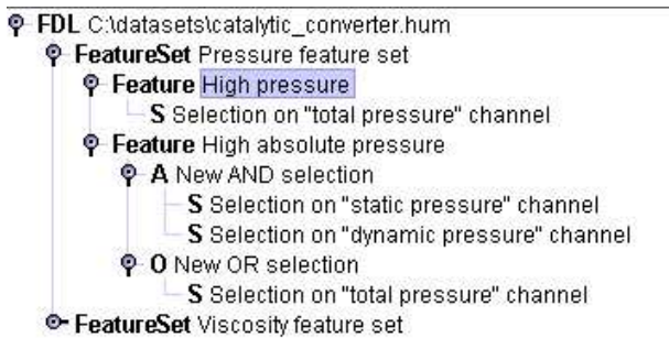
Figure 3: An example of FDL. The root node contains an arbitrary number of feature sets, which can be depicted simultaneously. A feature set contains one or more features logically combined of simple selections on data attribute ranges.
