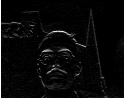
Fig. 6 – original image (top), image after application of Prewitt convolution filter (bottom)
