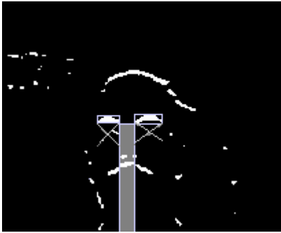
Fig. 8 – Edge image with recognized eyebrows and with area (filled with gray color) where to look for nostrils
