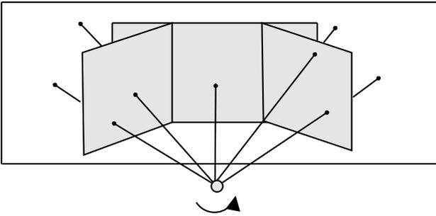
Figure 7: One image is selected as a reference, next homographies are computed for each neighboring image and finally all images are mapped to reference image plane [12]
