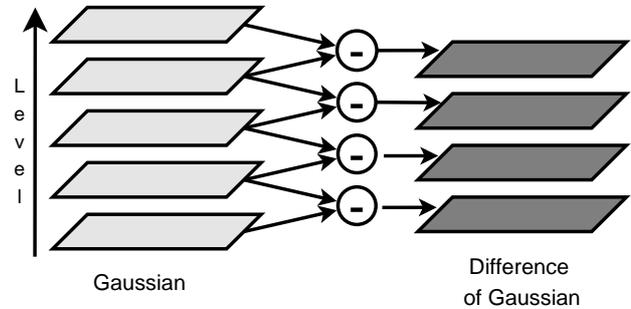
Figure 2: Adjacent images blurred with Gaussian function are subtracted to produce the DoG images [11].
