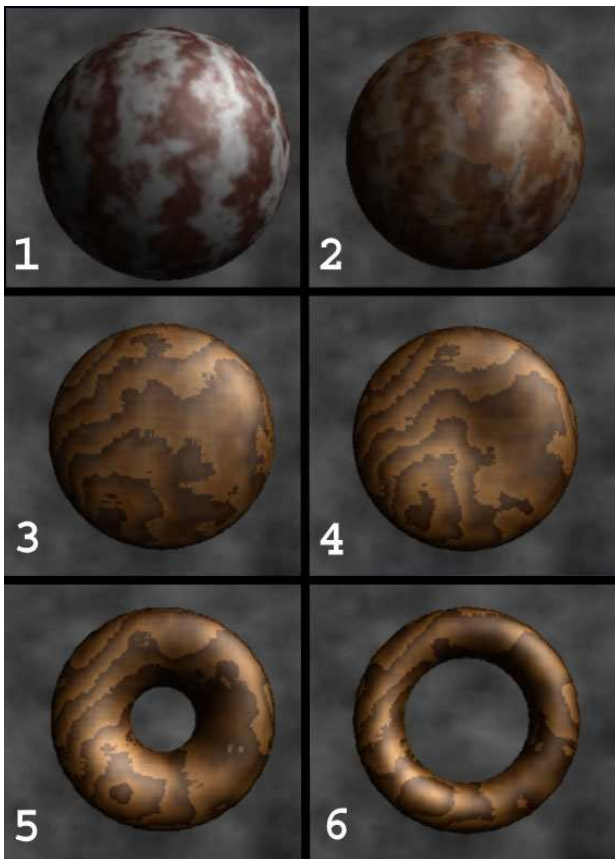
Figure 7: Smooth metamorphosis of two objects with different geometry and texture (no preprocessing here!). This kind of topology change is hard to carry out in the conventional vertex based modeling methods. The implicit modeling solves it by making the weighted sum of the interpolated modeling functions. 24 FPS, 1280×1024 (70 FPS without textures).
