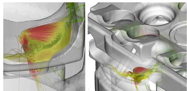
Figure 5: Detail and overview of a gasket vortex causing no problems. Now velocity magnitude is expressed with color. Red indicates fast swirling flow improving the cooling process.
