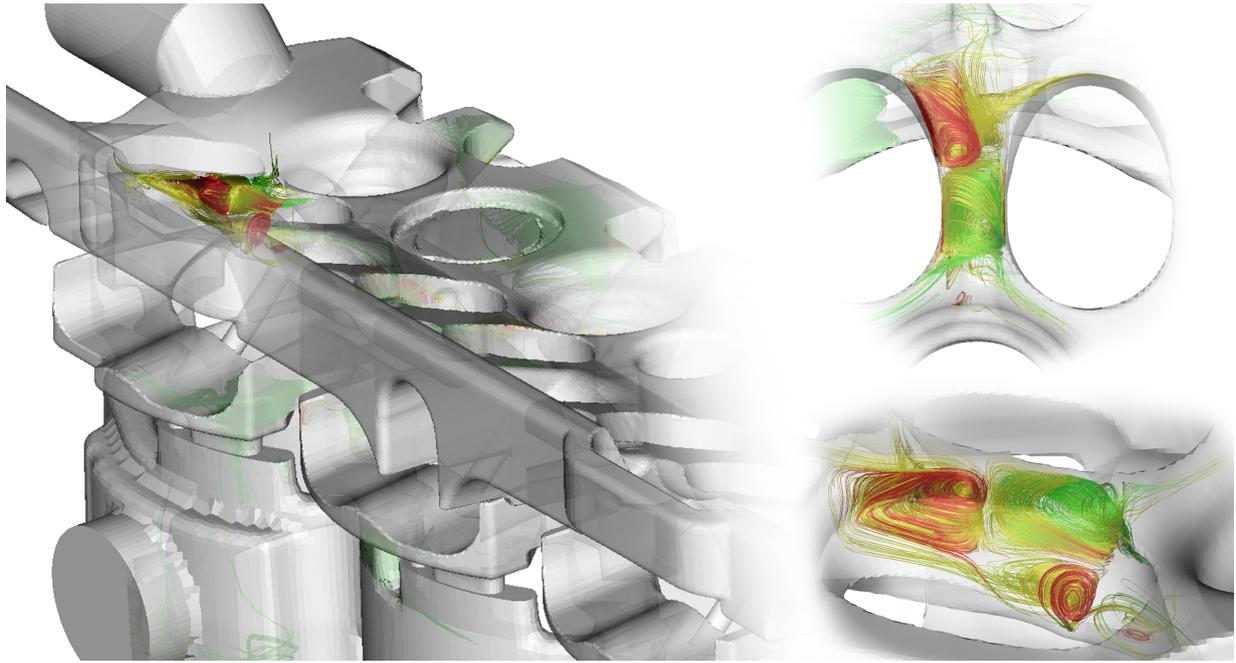
Figure 6: Visualization of an unwanted vortex with temperature mapped on the color of the streamlines. Critical values are shown with red, optimal with green. (left): An overview of the cooling jacket with a strong recirculation zone. Red color indicates overheating caused by blocked heat transport. (top): A top view of the recirculation zone caused by non-optimal jacked design. (bottom): We can recognize three separate vortices pushing against each other and conserving the flow.
