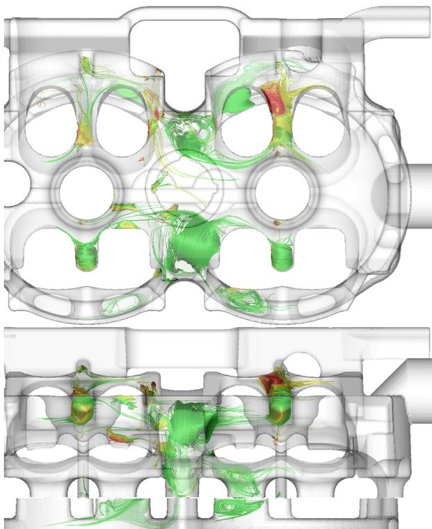
Figure 4: Overview of the recirculation regions around the fourth cylinder, top and side projection. Green regions symbolize low temperatures, red ones are critical. Most of the vortices are caused by the gasket connections, but in one region the fluid circulation causes overheating.
