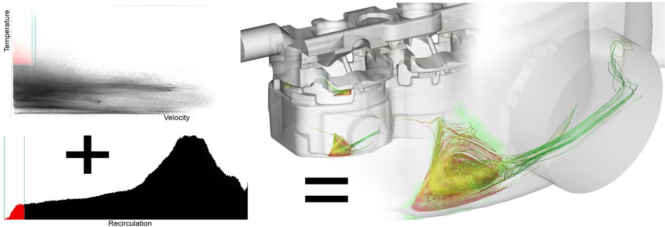
Figure 7: (top left): Brushing was used to select high temperatures and low velocities. (bottom left): Linked selection of recirculating line segments. The linked DOI displays only lines seeded in selected cells. (middle): Overview of the examined area under the outlet. (right): Detail of a recirculation zone delaying the cooling process displayed using a focus+context visualization. The temperature increases towards the center of the zone becoming red.
