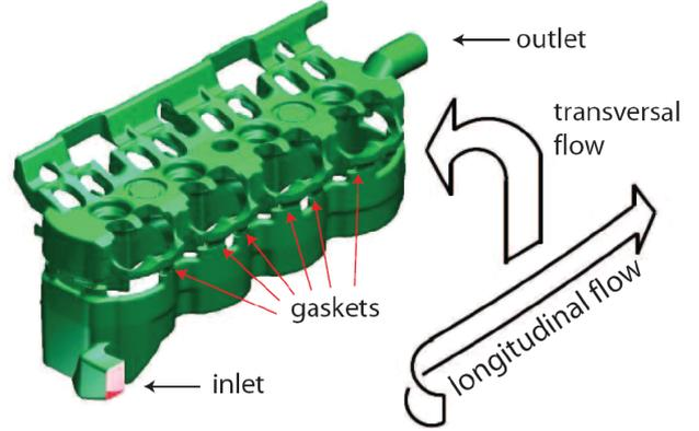
Figure 3: The major flow components inside of the cooling jacket include a longitudinal component from inlet to outlet and a traversal component in the upward-and-over direction through the gaskets. Image courtesy [8].
