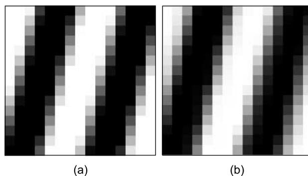
Figure 1: (a) Original pattern with 4 px thick synthetic lines 15 × magnified. (b) The same pattern resampled at scale 1.05 using bilinear interpolation. Note that edges of lines in the resampled image are significantly blurred.
