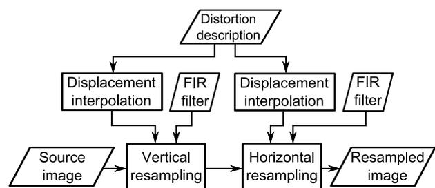
Figure 4: Dataflow of the resampling algorithm in FPGA.
