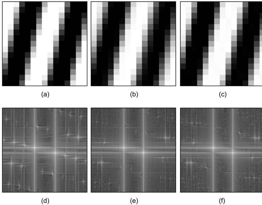
Figure 5: (a) Original pattern with 4 px thick synthetic lines  $15 \times$  magnified and (d) its power spectrum. (b) The same pattern resampled at scale 1.05 using bilinear interpolation and (e) its power spectrum. 88.96 % of energy of the power spectrum has been preserved. (c) The same pattern resampled at scale 1.05 using our proposed algorithm and (f) its power spectrum. 91.77 % of energy of the power spectrum has been preserved.
