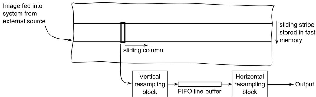
Figure 3: Overall processing of the image resampling.
