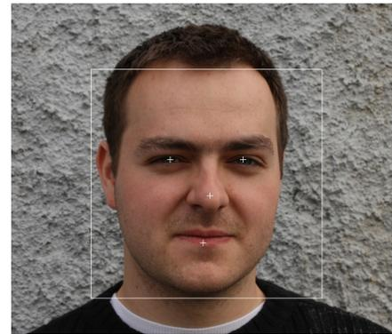
Figure 5: Face region and facial features detection by Haar Cascade Classifiers. Facial features are marked with a cross and face region with a rectangle.
