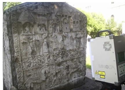
Figure 2: Scanning the stecak with a Minolta 910 laser scanner
