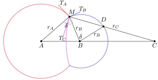
Figure 1: Geometry of bubble walls. Point  $C$  is the centre,  $r_c$  is the radius of the sphere which forms the common wall of sphere  $A$  and  $B$ .
