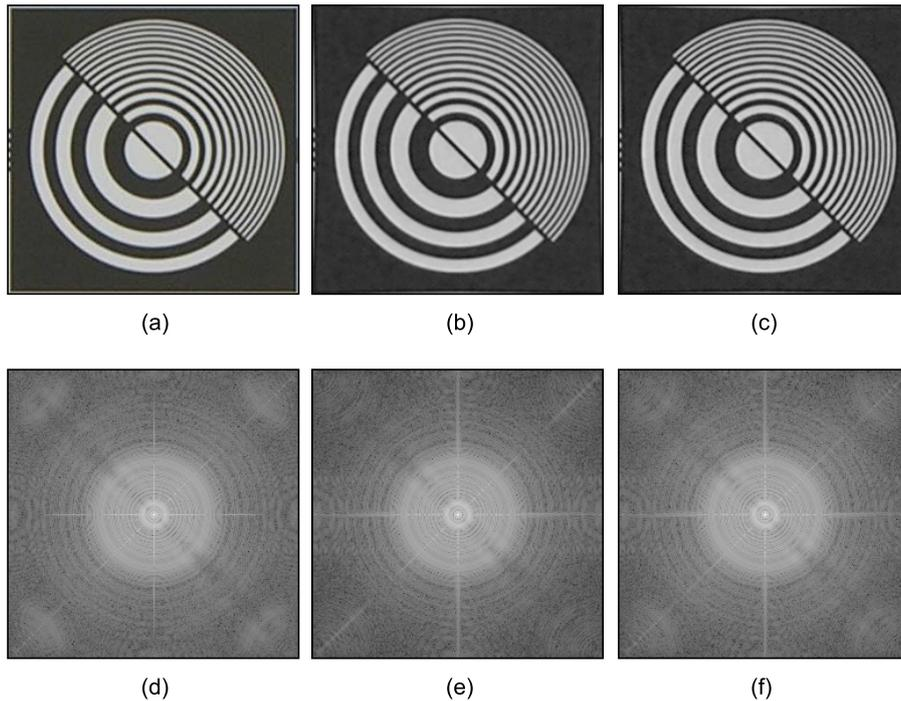
Figure 6: (a) Original image with a photographic pattern acquired by a camera and (d) its power spectrum. (b) The same image resampled using bilinear interpolation simulating barrel distortion correction and (e) its power spectrum. 90.32 % of energy of the power spectrum has been preserved. (c) The same image resampled using our proposed algorithm simulating barrel distortion correction and (f) its power spectrum. 98.45 % of energy of the power spectrum has been preserved.
