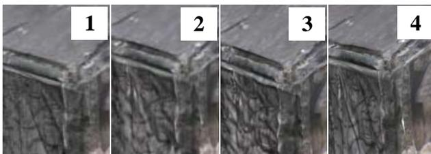
Figure 17: Comparison of models created by PP using Subdivide modifier: 1) created by Photomodeler (without post-modeling); 2) optimized with Subdivide “Size” parameter 1.5 (PP<sub>1</sub>); 3) maximum tested quality - Subdivide “Size” parameter 0.8 (PP<sub>3</sub>); 4) optimized for web - Subdivide “Size” parameter 4 (PP<sub>4</sub>)
