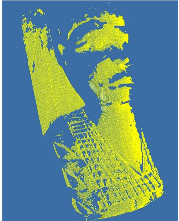
Figure 7: The final raw point cloud acquired from a set of 50 RGB pattern photographs.
