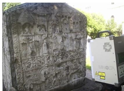
Figure 2: Scanning the stecak with a Minolta 910 laser scanner
