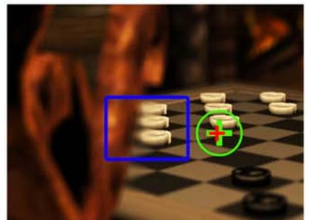
Top row: Example screens from our demo that present the resulting depth of field effect. Bottom row: The depth discontinuity problem (left) and the solution (middle) with its downside (right). On all figures the green crosshair represents the filtered, while red cross is the raw gaze point.
