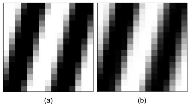
Figure 1: (a) Original pattern with 4 px thick synthetic lines 15 × magnified. (b) The same pattern resampled at scale 1.05 using bilinear interpolation. Note that edges of lines in the resampled image are significantly blurred.
