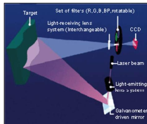
Figure 3: Minolta Vivid 910 measurement principle
