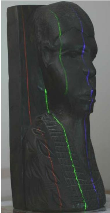
Figure 4: The RGB light pattern projected on the object.
