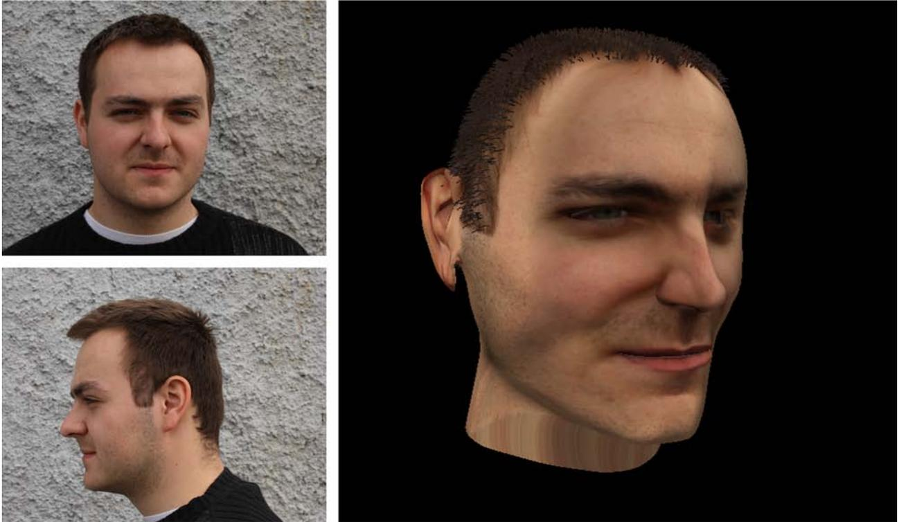
Example of source photographs (Left) and the reconstructed 3D head model (Right) rendered with the texture-space diffusion technique.
