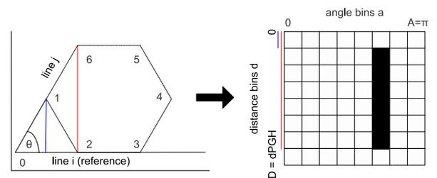
Figure 5: PGH computation of a single line
