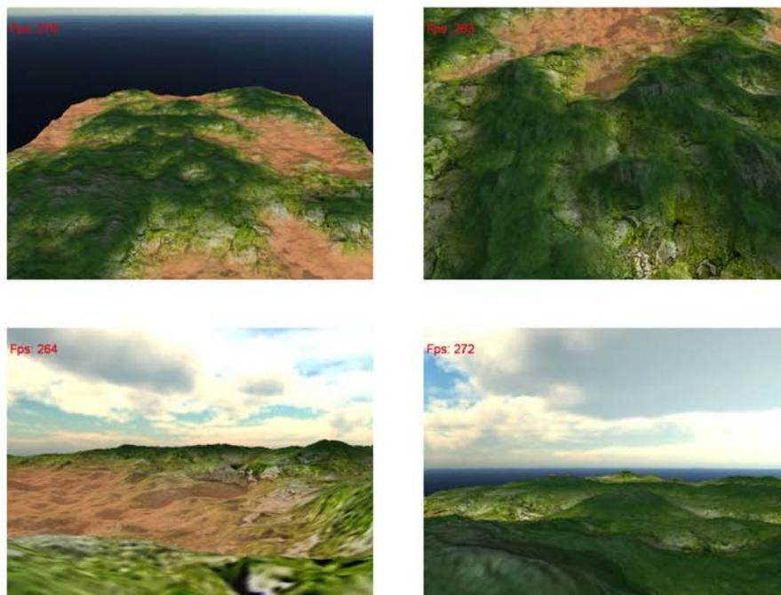
These four viewpoints were selected to be used during frame rate test of the algorithm on different platforms with different options. Shown frame rates were achieved on Geforce 8800 GT, 2049 × 2049 height map, 256 × 256 quads.
