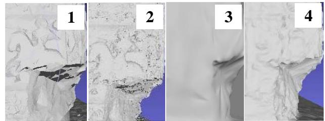
Figure 19: Geometry quality comparison: 1) optimized LS model for web purpose (LS<sub>3</sub>); 2) non-optimized LS model (LS<sub>1</sub>); 3) optimized PP model for web purpose (PP<sub>4</sub>); 4) maximum quality PP model (PP<sub>3</sub>)
