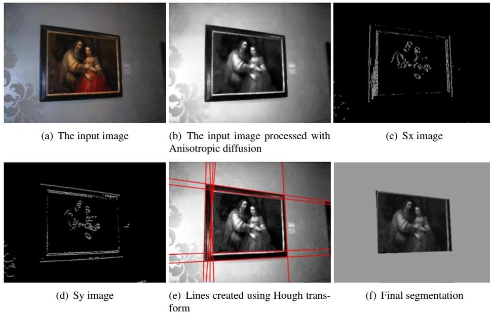
Figure 4: The process of the Anisotropic diffusion method of the segmentation.
