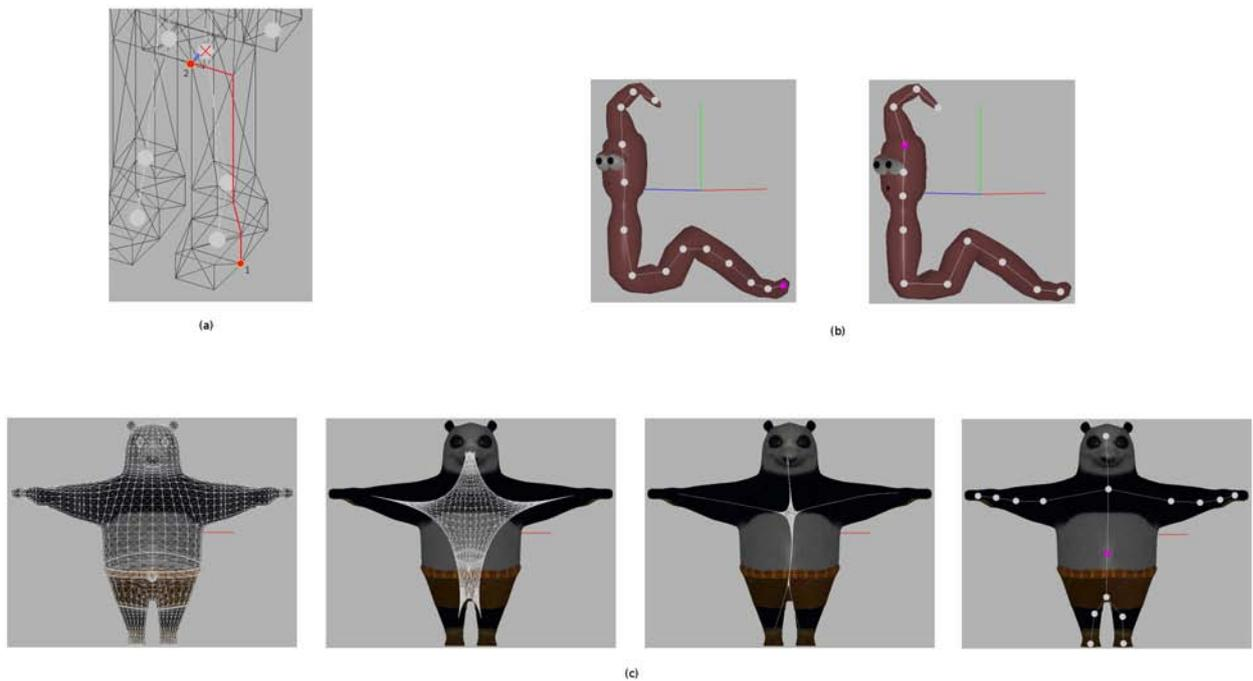
(a) Computation of the geodesic distance between the control point marked with red cross and the mesh vertex. (b) Comparison of the extracted skeleton (left) and the skeleton rigged by an artist (right). (c) Example of the contraction of the geometry and the extracted skeleton.
