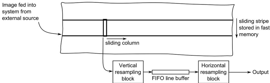
Figure 3: Overall processing of the image resampling.
