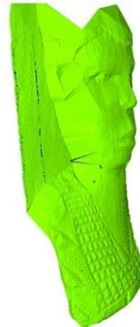
Left: A photograph of a sample plate of the Wkryjście Altar titled: Jesus Christ coronation with thorn. Middle: The test object used to prototype the reconstruction technique. Right: The final mesh reconstructed from the point cloud.
