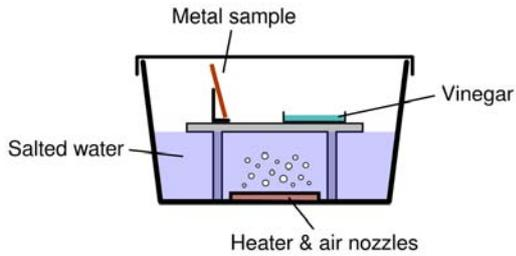
Figure 4: Our setup to accelerate the rusting process between measurements.
