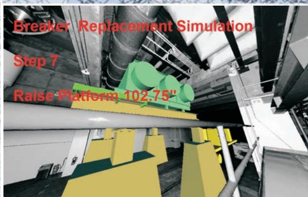
Simulate equipment removal / replacement with 3D animation. Verify for clash detection.
