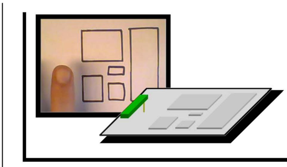
The system is able to recognize a hand drawn keyboard and compute a position of the finger in the space.
