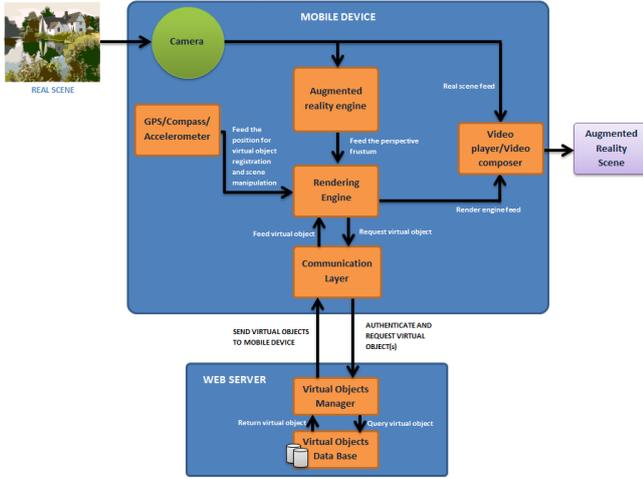
Figure 3.1 AR Mobile Platform architecture
