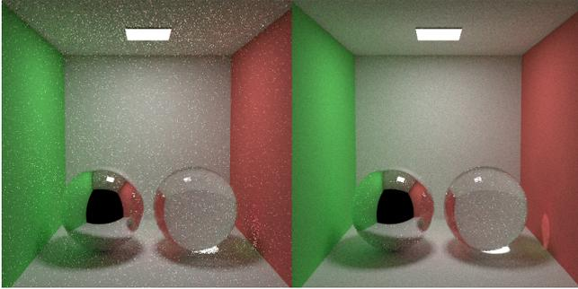
Figure 2: Difference between path tracer and bidirectional path tracer when computing caustics. On the left side, the fireflies generated by standard path tracer compared to more smooth caustics generated by the bidirectional path tracer on the right side.
