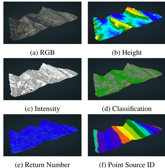
Figure 1: Coloring different point cloud attributes; CA13 point cloud courtesy of [8]
