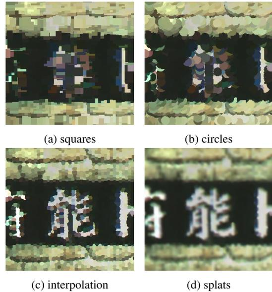
Figure 4: 4 different rendering modes. Squares and circles have issues with overlapping points. Interpolation and splats provide considerable improvements in readability of high frequency features. Point cloud courtesy of [11]
