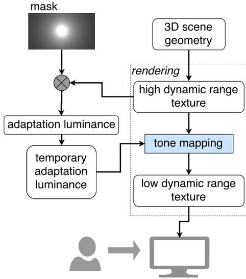
Figure 4: The diagram of the visual adaptation module.
