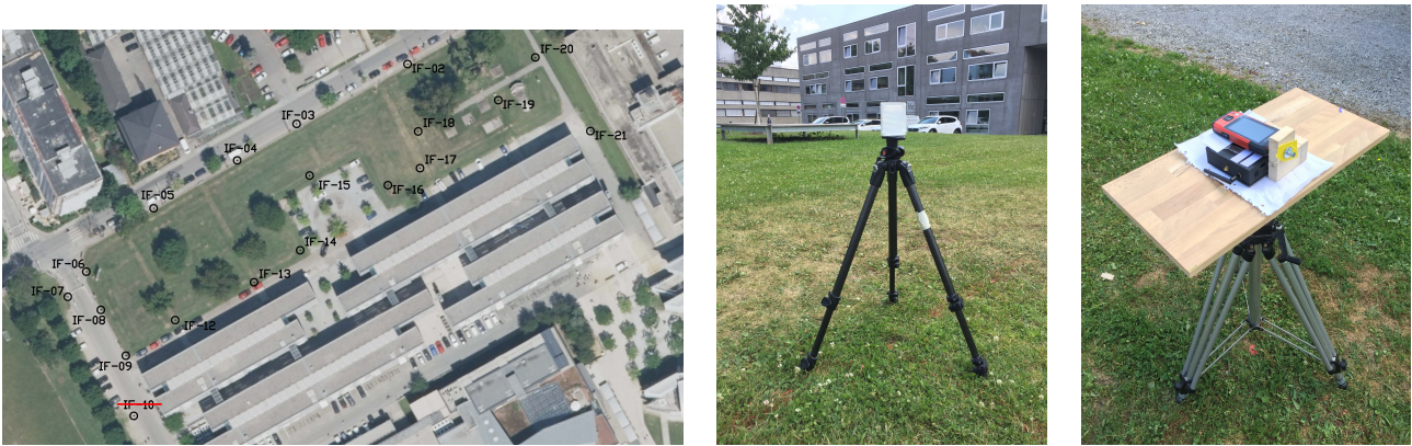
Figure 4: Environment setup for the compass validation. Left: Map of all reference Points. Middle: Reflective prism on a tripod. Right: Laser Range Finder mounted on the sensor cube.
