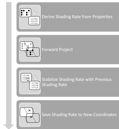
Figure 5: The core steps executed in the compute shader of our STeFAS algorithm. First, the shading rate is derived from the clipping distance. In the next step, the coordinates in the next frame are computed by a forward projection. Finally, the shading rate is stabilized by our TAA-based approach and saved to the new coordinates.
