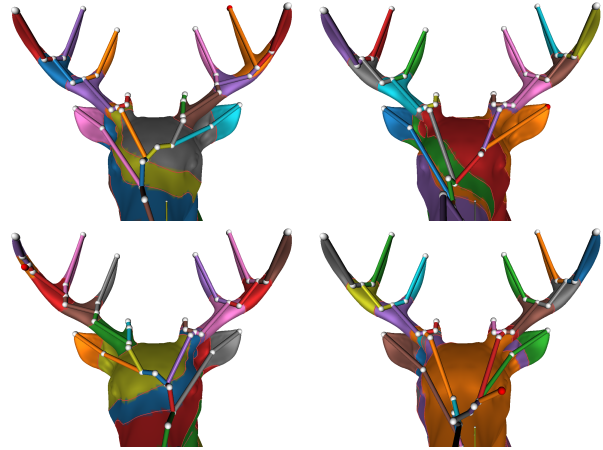
Figure 8: Natural Reeb graphs embedded into the mesh. Each example has a different start vertex highlighted in red.
