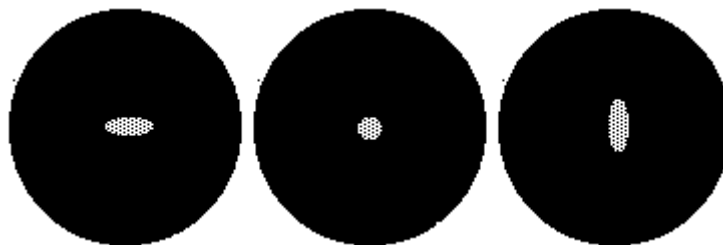
Figure 5: Astigmatism aberration, from left to right : inside focus, best focus, outside focus.
